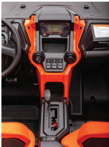
Honda's DCT allows drivers to select between two fully automatic modes — Drive and Sport.
