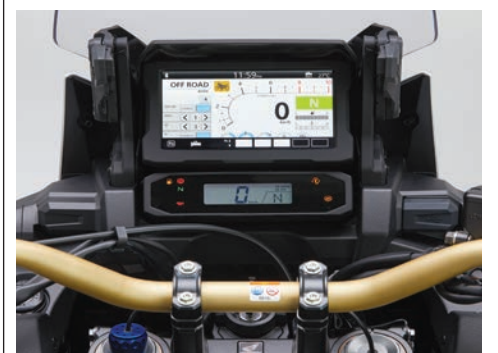
A full-color 6.5-inch TFT color touchscreen allows for a variety of rider input.
