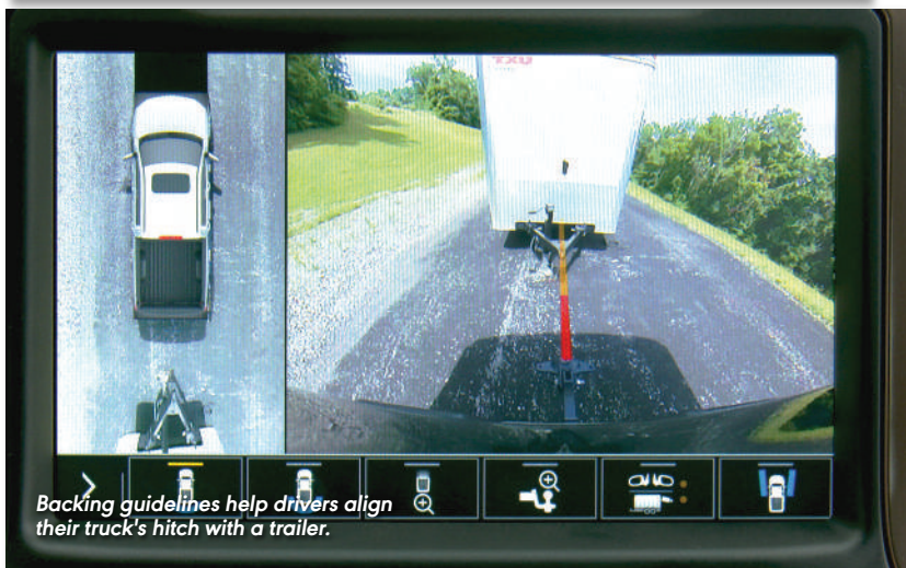
Chevy's ATS package uses cameras that provide a 270-degree view.
