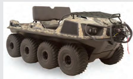
The 2021 Aurora 800 Huntmaster features a front rack, winch and rear cargo box as standard equipment. Photos courtesy of ARGO
